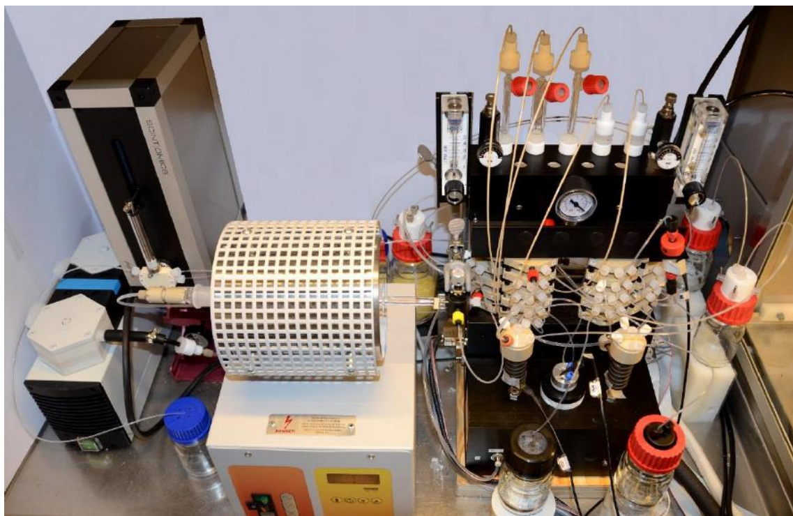
Figure 1. The automatic equipment for astatine recovery from target material and subsequent carrier labeling
