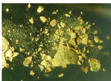
Figure 1 – Precipitate found in T4 column.
