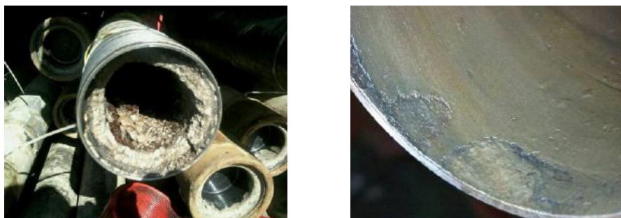
Figure 1 Mineral scale, mainly barite (left) and metallic lead (right) on oil tubulars
