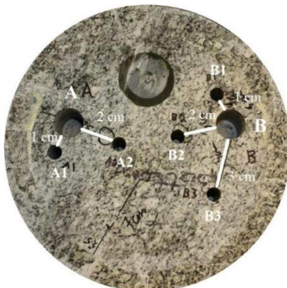
Figure 1. Grimsel Granodiorite rock block used in in- and through diffusion experiment.
